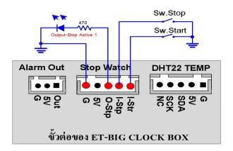
In this case, Input that is connected to Pin I-Str is used as Switch Start Timing; and Input that is connected to Pin I-Stp is used as Switch Stop Timing. Both Inputs are Pull-Up inside at 5V; so, it has to send Logic '0' to control Start or Stop instantly; in this case, format of Signal Logic '0' should be Trig as the same as Push-Button Switch.
